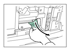
**10** Replace the MP transport tray in its original position, then close the front cover.
